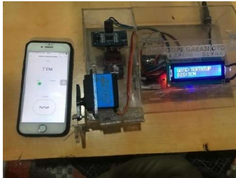
Fig. 1. Automatic door latch control system
