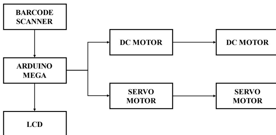
Fig. 1. Hardware design block diagram
