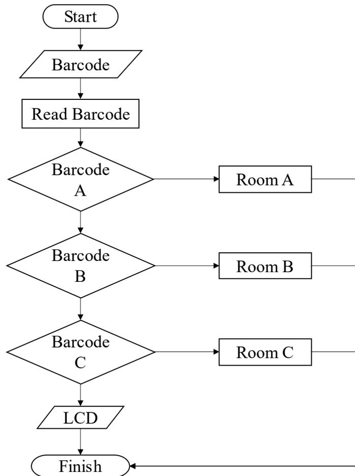
Fig. 2. Flowchart of beam package separation system
