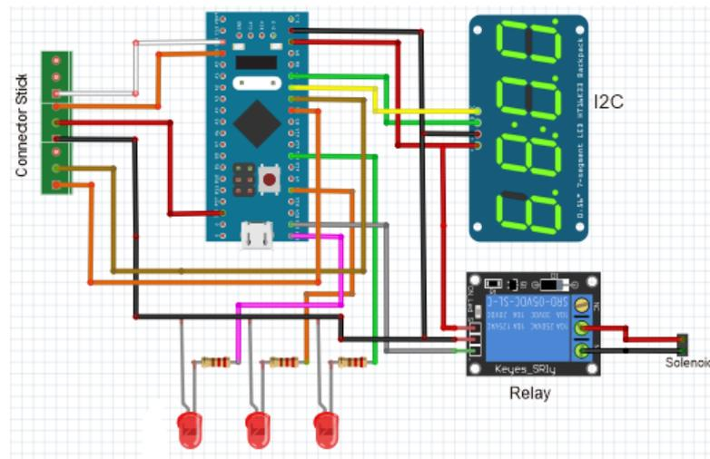
Fig. 4. Wiring circuit
